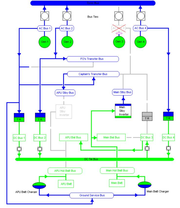
Electrical fault: AC Bus 3 failed
